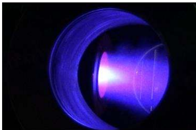
Figure 1. Operation of rotating arc reactor using H 2 /Ar mixture.
